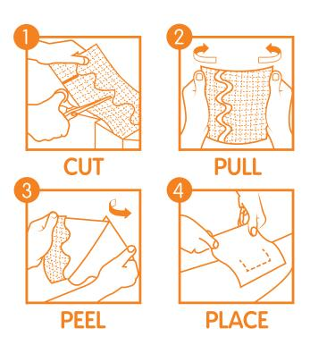
The grid pattern facilitates measurement and cutting of the required length, ensuring easy and safe application.
